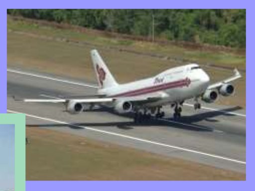
Boeing 747-400 Length: 70.6 m Span: 66.4 m Height: 19.4 m
