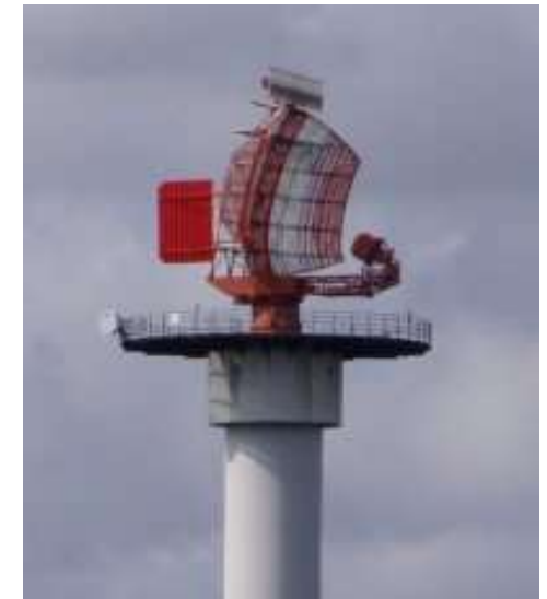
↑ Monopulse Mode S PSR + MSSR
