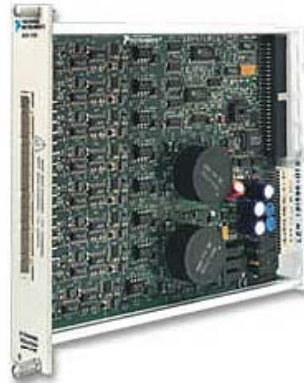
NI SCXI-1125: 8-Channel Isolation Amplifier
